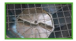
The integrated mixer in the material hopper effectively prevents the formation of "bridges" with very light materials. Additionally, the mixer contains strong magnets that can largely remove potential foreign objects such as nails or metal shavings.
