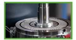
High-quality hardened flat dies available for various pellet diameters and different press channel lengths.
