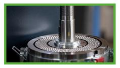
At the heart of the pelletizing process are specially hardened flat dies available in various pellet diameters and press channel lengths.
