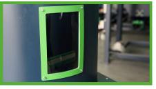
The dosing system features sight glasses on both sides for visual level monitoring. Additionally, a sensor alerts when the fill level falls below 30%.
