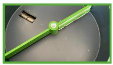
An internal agitator prevents the formation of blockages and ensures a consistent material flow.
