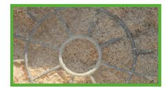
The mixer located in the material hopper prevents possible "bridging" of very light materials. Furthermore, strong magnets are integrated on the mixer, which can sort out possible foreign bodies such as nails or metal chips.
