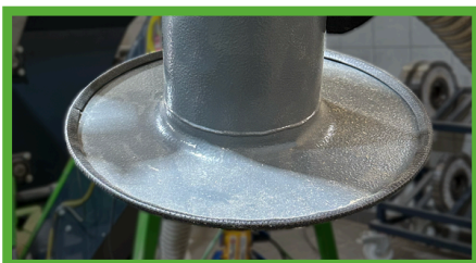
Point extraction with at least 10 - 15 cm distance to the dust source
